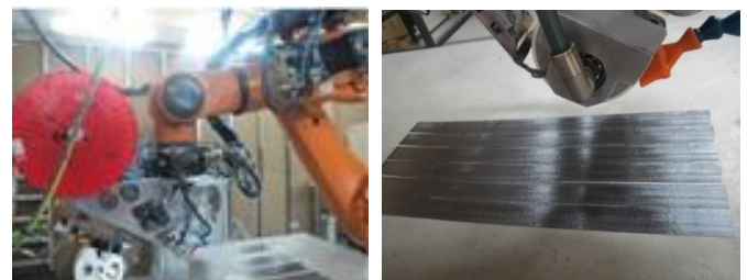
Figure 2. Automatic laser - assisted of UD1 and UD2 tape laying with machine manufactured by Mikrosam AD
