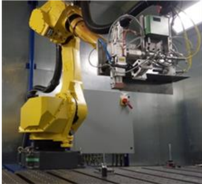
Figure 3 : Laser overlap welding setup
