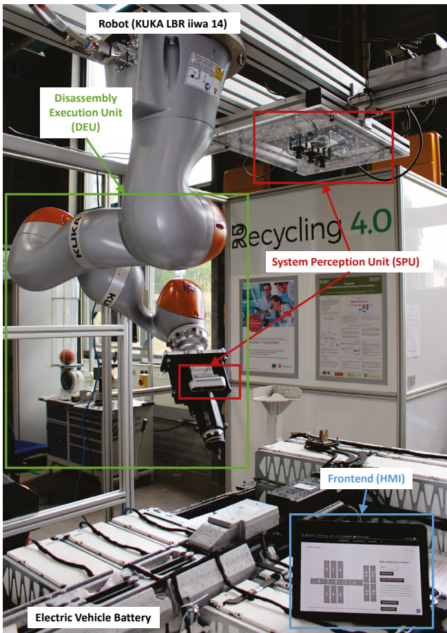
Fig. 4. Case study scenario on electric vehicle battery disassembly
