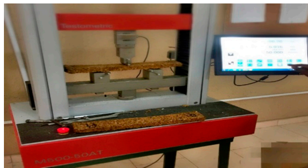
Fig. 2 Particleboards during flexural strength test
