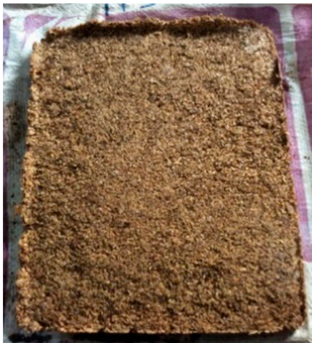
Fig. 1 Particleboards after moulding
