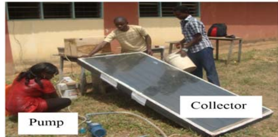
Plate 1: The arrangement of Active system while in operation
