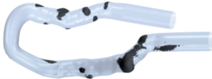
Figure 7.2: Isosurface of flow recirculation (negative streamwise velocity) in all four cases.
