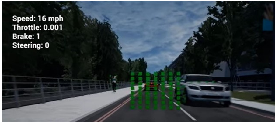
Figure 6: Faking lidar signals in a vehicle simulation (WMG image)
