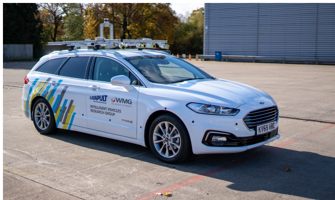
Figure 8: WMG’s drive-by-wire HVM Catapult innovation platform vehicle (WMG image)
