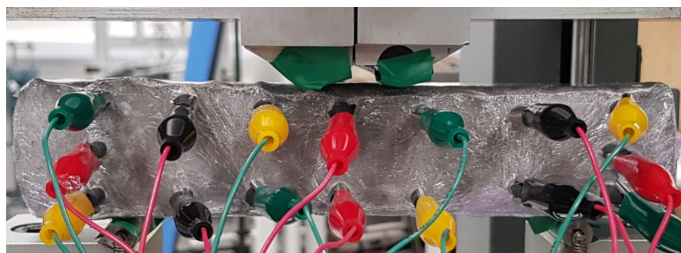
Figure 7. Small-scale beam bending experimental setup, with 16 electrodes interrogating an AAM patch on the concrete surface. Green tape was used to insulate the loading machine from the sample.
