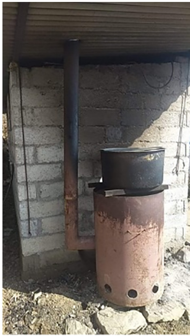
Fig. 7. TLUD condition in 2020 after 2 years of use - Buddhist Retreat Centre P5 (colour).
