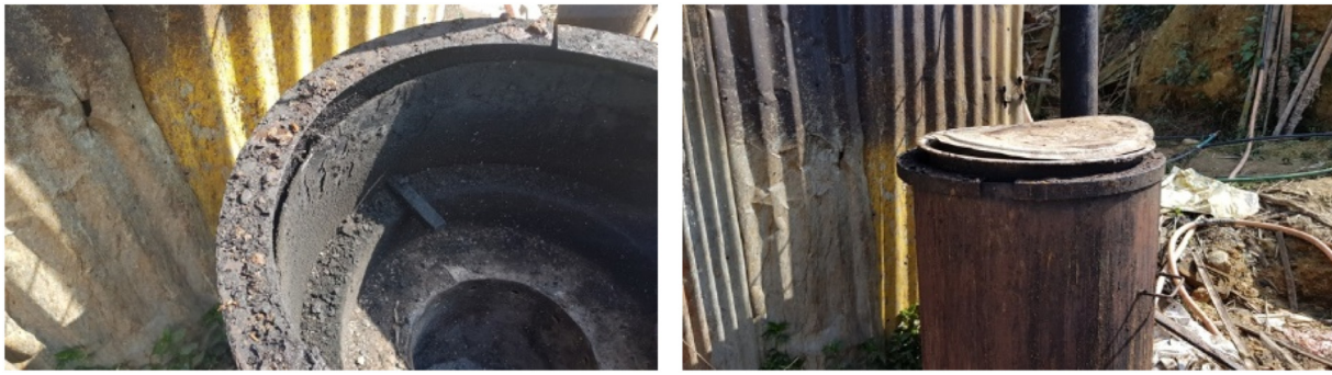
Fig. 6. TLUD condition in 2019 after 1 year of use - study site 1 - P3 - small dairy farmer (colour).
