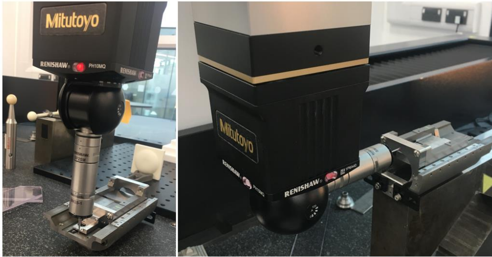
Figure 20. CMM measurements for the verification of the KCs.
