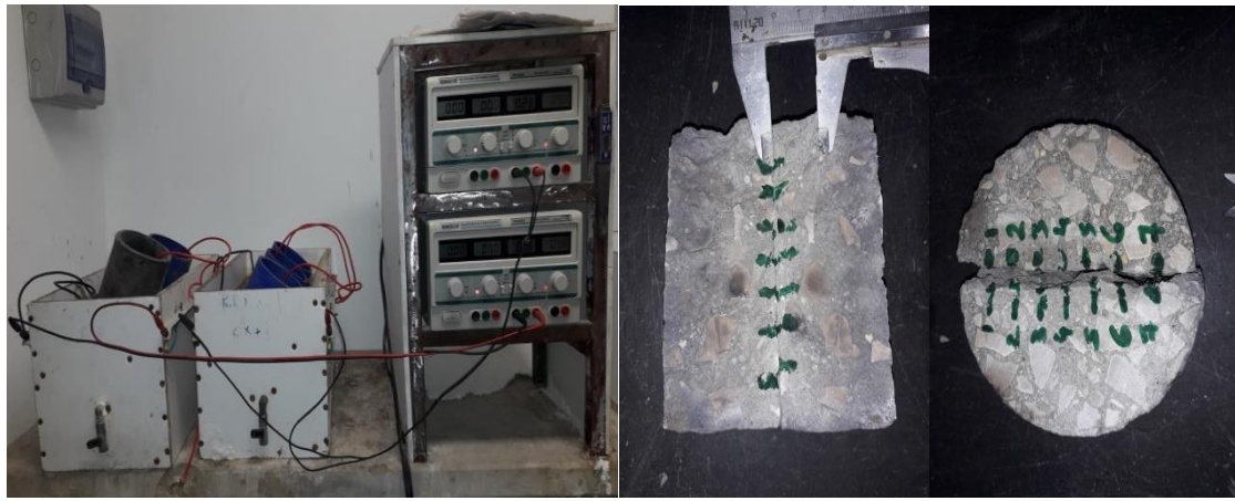
Figure 4.5: The picture on the left (a) is for the RCPT machine and on the right (b) is for a broken sample while measuring the depth of chloride penetration
