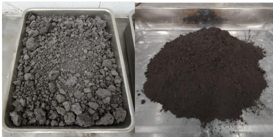
Figure 4.2: A picture showing the EAFS as-received (a- left) and after milling to the required size for use as a precursor in concrete (b-right)
