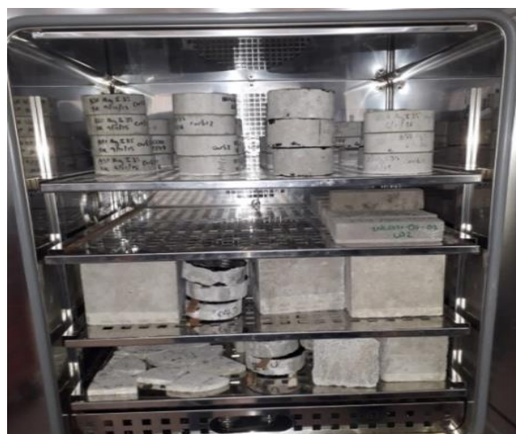
Figure 4.6: Samples in the carbonation chamber
