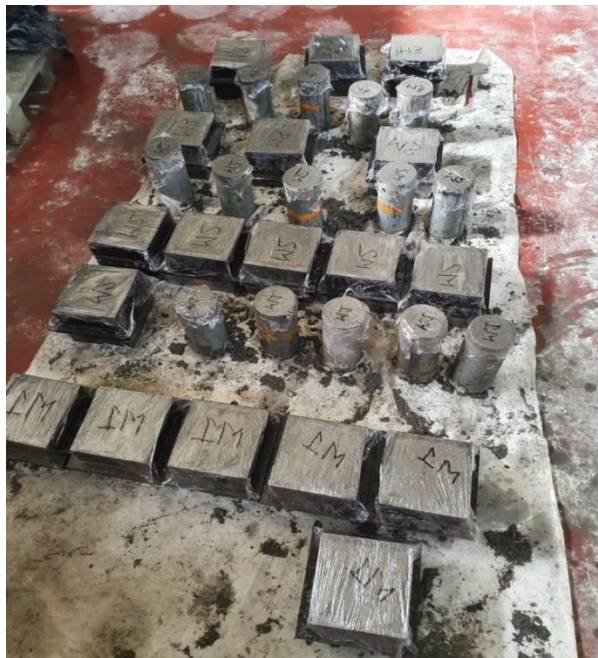
Figure 4.4: A picture of the casted AAC samples with the plastic wrap prior to thermal curing
