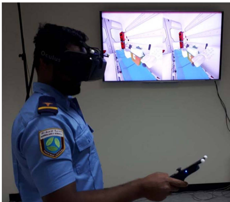
Figure 1. Paramedic interacting with the VR setting via the Oculus Rift DK2 head-mounted display and hand-held controller to grip and move objects.
