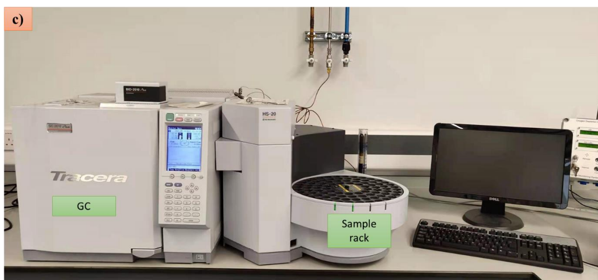
Figure 1.24 Workflow for high-throughput screening: (a) Swing by Chemspeed Technologies; (b) Solar simulator (AM1.5G, Class AAA, IEC/JIS/ASTM, 1440 W xenon, 12 × 12 in., MODEL: 94123A) with rocker/roller device; (c) HS-20 GC System.
