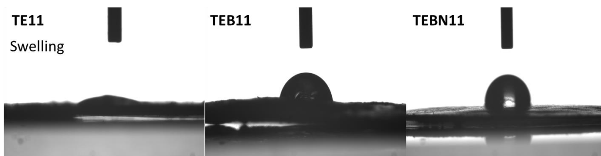
Figure 2.27 Contact angle images against water of TE11, TEB11 and TEBN11. For swelling polymer TE11, the image is taken several seconds after the drop is deposited onto the polymer surface.
