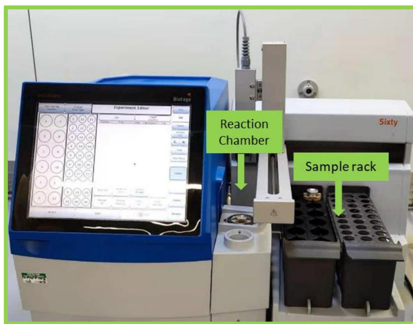
Figure 1.26 Automation for microwave assisted organic synthesis, Biotage Initiator + microwave system.
