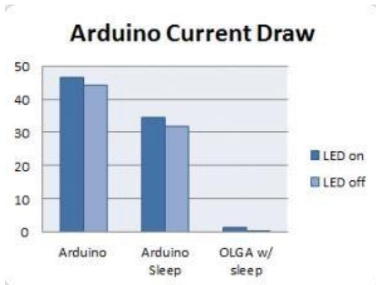
Figure 20. Comparison of the results between Arduino pro mini and the customized board[64].
