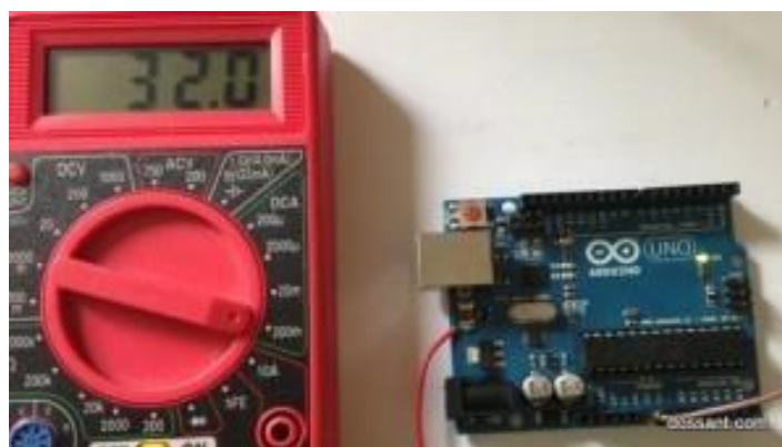
Figure 17.A Multimeter displays the actual measured current consumption when the Sleep Code is deactivated and Power LED is off [64].
