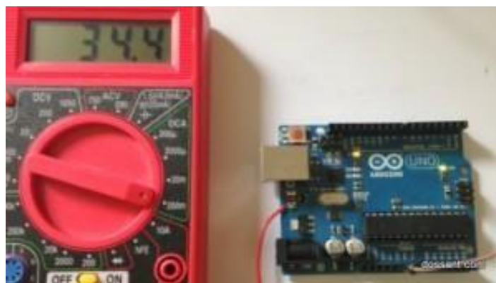
Figure 16.A Multimeter displays the actual measured current consumption when the Sleep Code is activated and Power LED is on [64].
