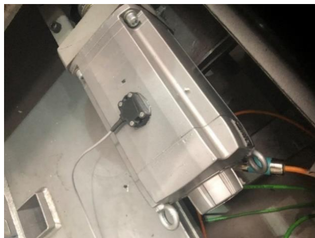
Figure 10. ADXL355 MEMS used to measure the vibration [60]
