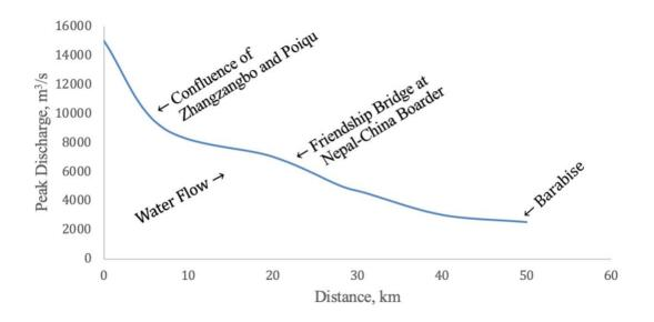
Figure 3.15 GLOF from the Zhangzangbo Glacial Lake, Poiqu River, Tibet (China) or the Bhote (Sun) Koshi (Nepal), Peak discharge attenuation downstream, (Modified from Xu Daoming, 1985)
