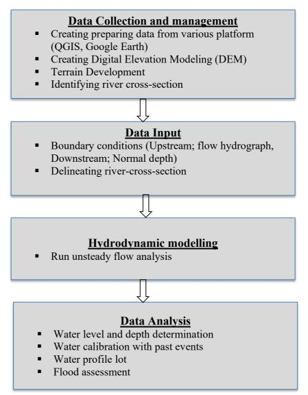
Figure 3.3 Data processing and HEC-RAS modelling
