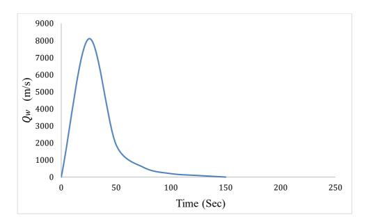
Figure 3.6 Calculated breach hydrograph
