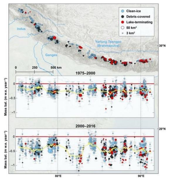
Figure 2.5 Map of glaciers and mass balance at HKH region. Glacier areas are proportional to circle size, colour shows clean-ice, debris-covered, and laketerminating categories. Insets indicate ice loss during 1975 to 2000 and 2000 to 2016. (Maurer et al., 2019).
