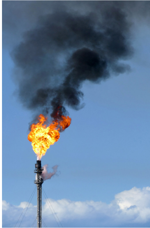
Figure 3: Gas flare on an elevated stack. Due to incomplete combustion, significant amount of soot is being released in the form of smoke. Image source: Wikipedia Commons (Carter n.d.).
