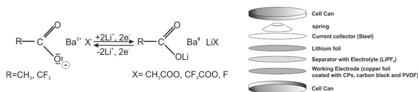
Scheme 1. Lithium storage mechanism of CP at molecular structure level and schematic structure of the LIBs.
