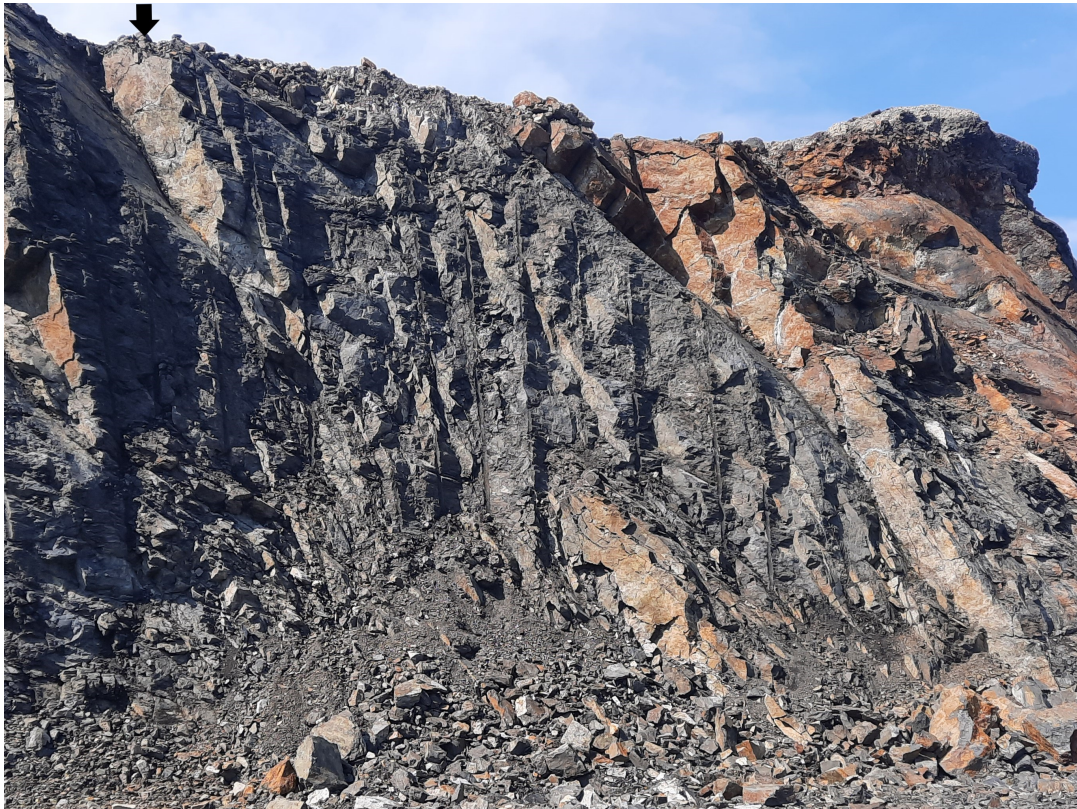
Figure 30: A more detailed photo of the presplit face from the left side of figure 28. The black arrow functions as a reference point between figures 28 and 29.
