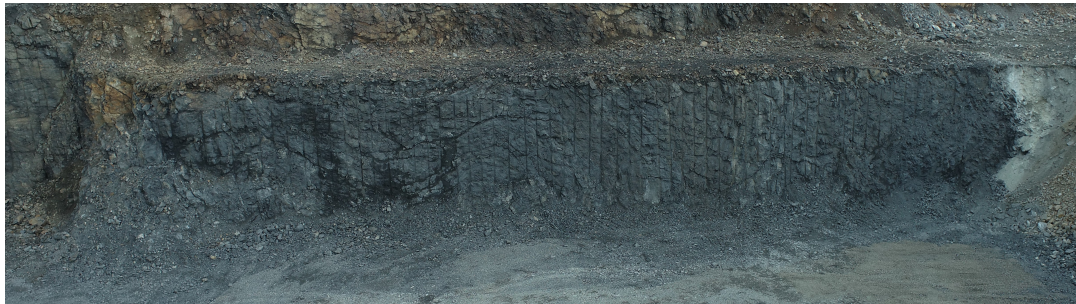
Figure 35: Photo of the second black schist test presplit face (BS 2.1).
