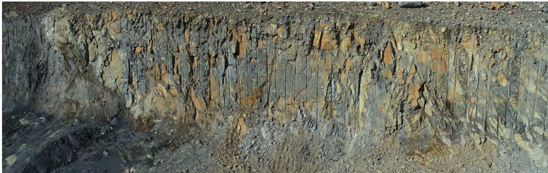
Figure 25: First part of the presplit test after scaling (MS 2.1).
