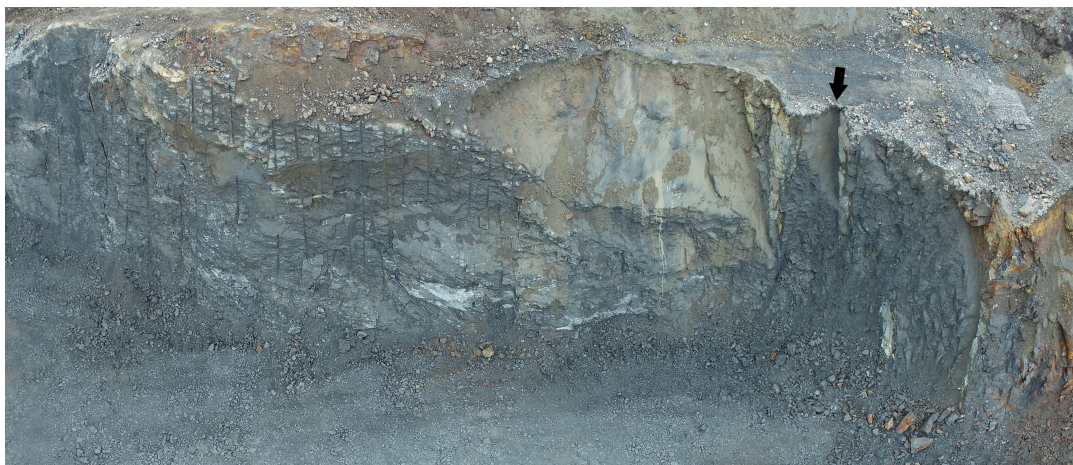
Figure 29: Photo showing an overview of the first part of the presplit wall in the first test in black schist (BS 1.1). The black arrow functions as a reference point between figures 28 and 30.
