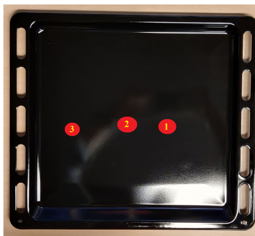
Figure 5.7: Placement of thermocouples in oven tray
