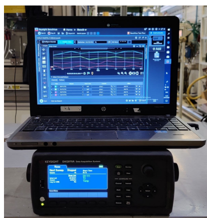
Figure 5.10: Keysight DAQ970a data acquisition system
