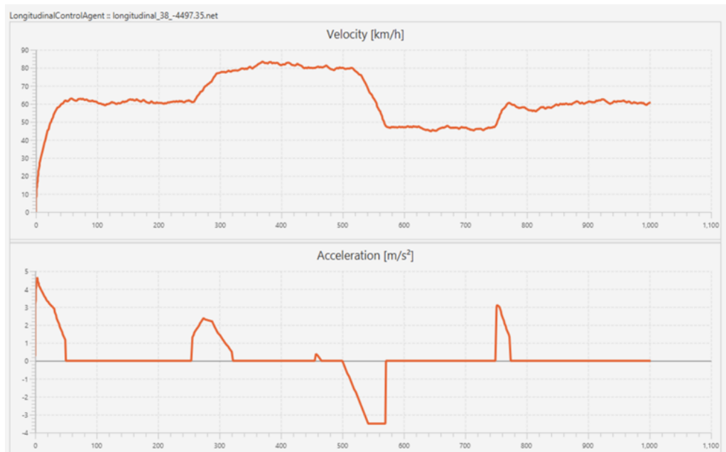
Figure 19. Velocity and Acceleration performance on noise tolerance. Extracted from Cooperative Traffic Simulator.
