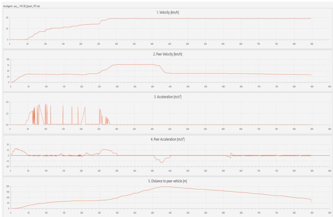
Figure 40. Velocity, PeerVelocity, Acceleration, Peer Acceleration, Distance to peer vehicle for 5 actions. Extracted from Cooperative Traffic Simulator.
