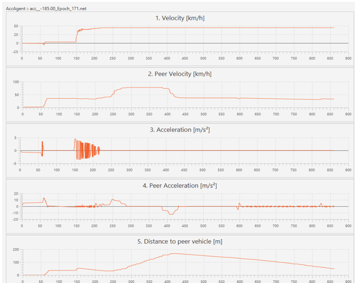
Figure 39. Velocity, Peer Velocity, Acceleration, Peer Acceleration, Distance to peer vehicle for 4 actions. Extracted from Cooperative Traffic Simulator.
