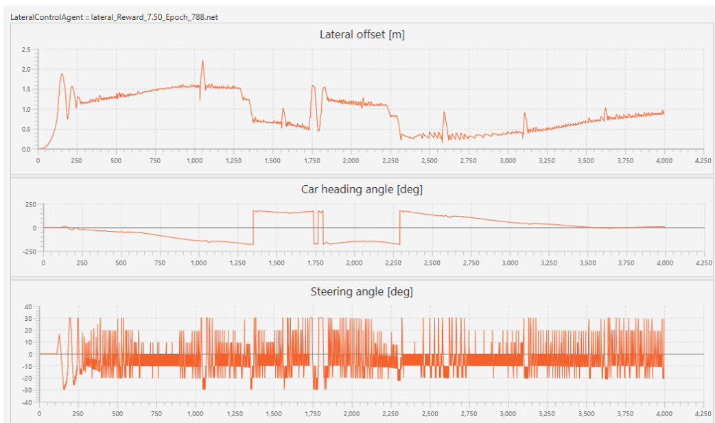
Figure 33. Lateral offset, Car heading angle, Steering angle of 4 actions for the second track. Extracted from Cooperative Traffic Simulator.
