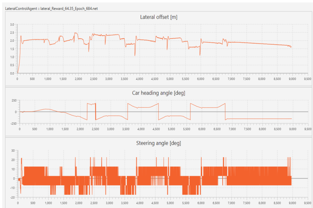
Figure 37. Lateral offset, Car heading angle, Steering angle of 5 actions for the second track. Extracted from Cooperative Traffic Simulator.
