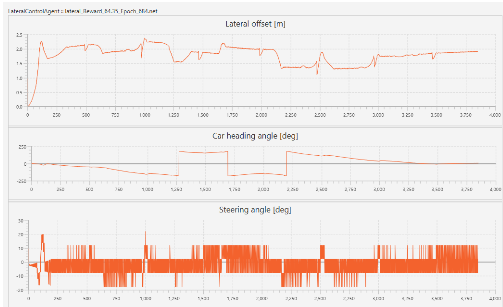
Figure 37. Lateral offset, Car heading angle, Steering angle of 5 actions for the second track. Extracted from Cooperative Traffic Simulator.
