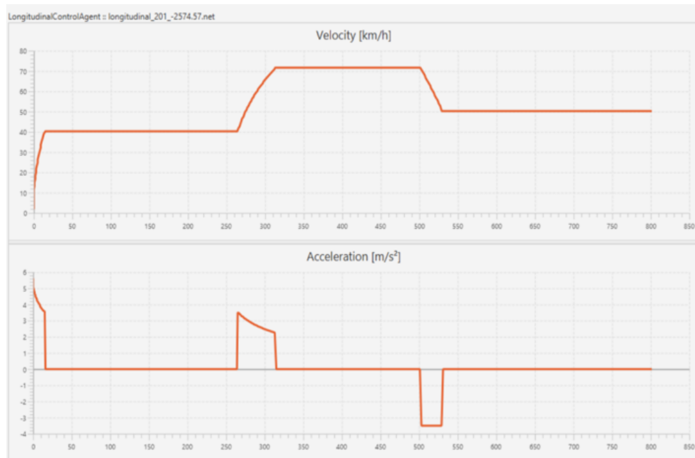
Figure 21. Velocity and Acceleration performance on different track length and speed limits. Extracted from Cooperative Traffic Simulator.
