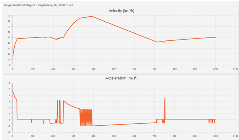
Figure 15. Velocity and Acceleration performance of 3 actions. Extracted from Cooperative Traffic Simulator.
