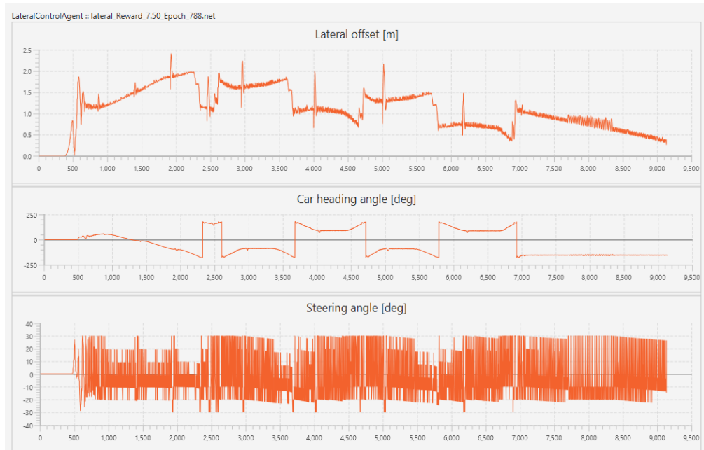
Figure 34. Lateral offset, Car heading angle, Steering angle of 4 actions for the third track. Extracted from Cooperative Traffic Simulator.
