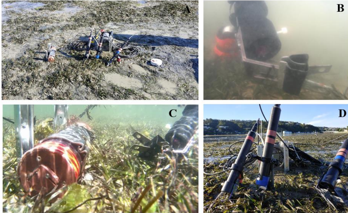
Figure 7.4: Moni-DA Diving PAM (Walz, Germany) along with ECOPARs deployment in the field. B & C) underwater detail of the deployment of the leaves in the clips of the instrument.
