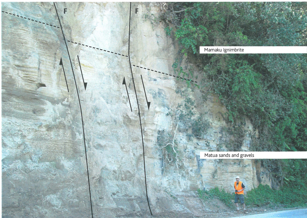
Fig. 17 Normally faulted planar-bedded Matua Subgroup sands, gravels and silts, overlain by massive pinkish-brown Mamaku Ignimbrite. Roadcut on Little Waihi Road (V14/162765).
