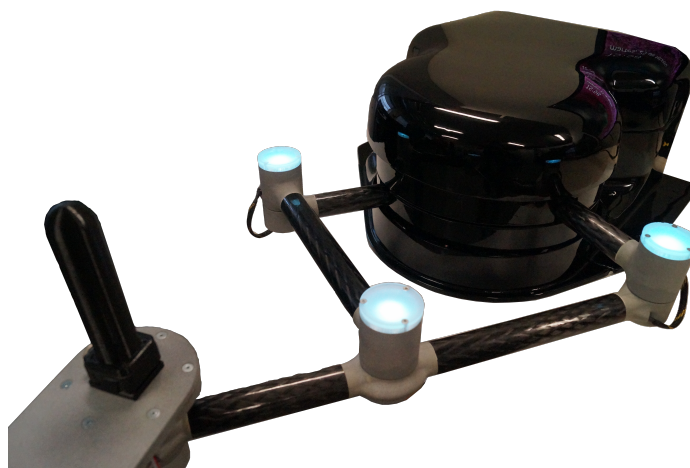
Figure 1. Upper-limb rehabilitation robotic device called Rubidium. Rubidium is commercialized and distributed by the spin-off iDRhA.
