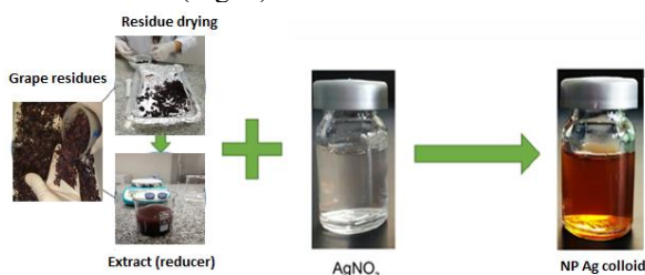
Fig. 1. Biosynthesis protocol of silver nanoparticles.
