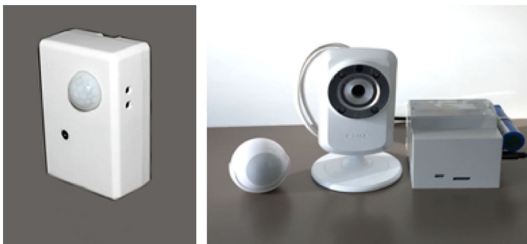
FIGURE 3 Left: Integrated version of the iCareBot based on raspberry pi 2. Right: iCareBot based on raspberry pi 3 with standalone motion sensor and webcam [Colour figure can be viewed at wileyonlinelibrary.com ]
