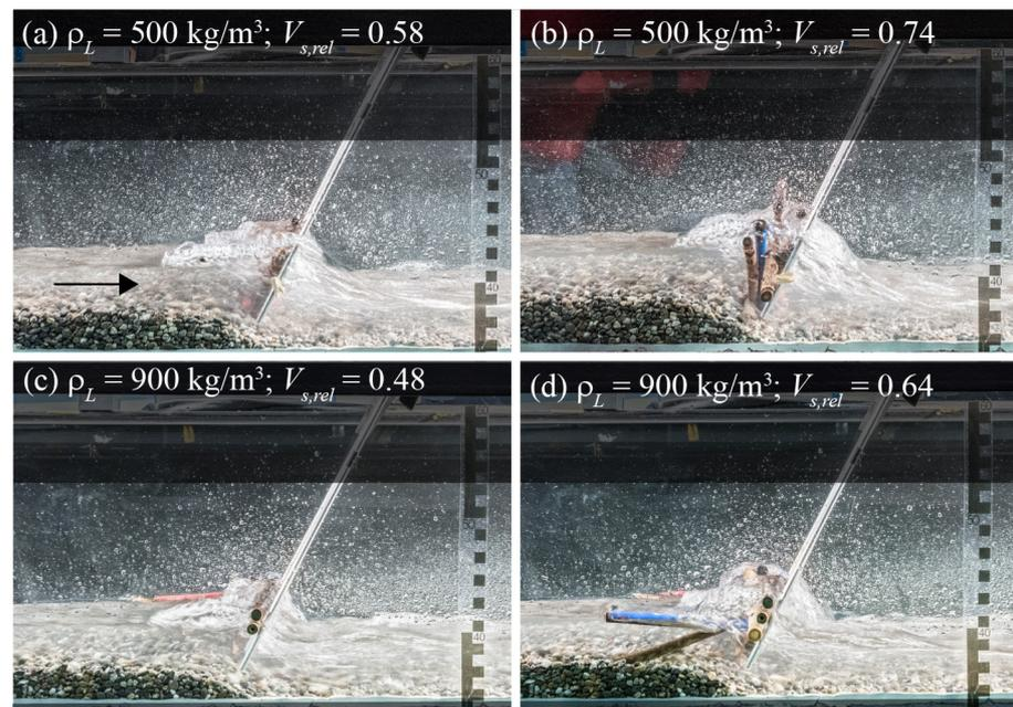
**Figure 4.** LW accumulation and bedload deposition at the inclined bar screen for (a) test V1b ( $\rho_L = 500 \text{ kg/m}^3$ ) with  $V_{s,rel} = 0.58$  and (b)  $V_{s,rel} = 0.74$ , compared to (c) test V4 ( $\rho_L = 900 \text{ kg/m}^3$ ) with  $V_{s,rel} = 0.48$  and (d)  $V_{s,rel} = 0.64$ .
