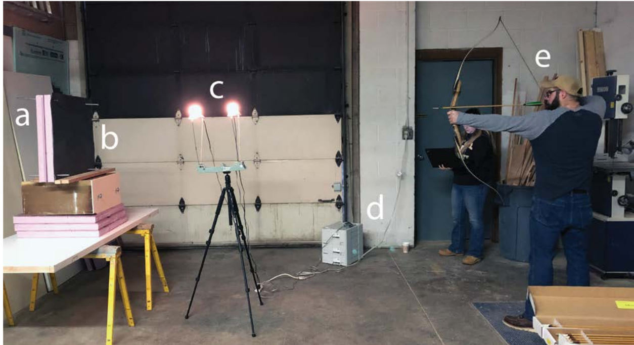
Figure 2. The experimental set up included two layers of two-inch-thick (5.08 cm), medium-density construction foam-board (a) covered by a sheet of 8oz vinyl Naugahyde (b). Arrows were shot through a chronometer (c) so velocity could be recorded (d). M.W. used a recurve bow to shoot the arrows approximately three meters from the target (e).
