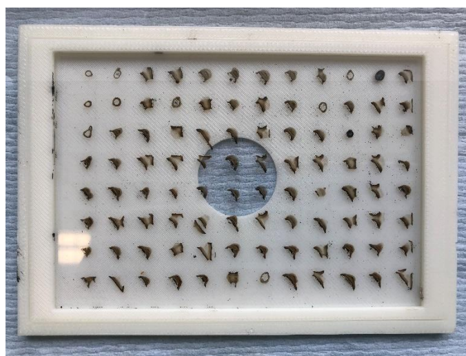
Figure S4.22: The immobilised \text{Co}_3\text{O}_4 -MMO catalysts on the glass plate, after treatment of the glass plate with the piranha solution.
