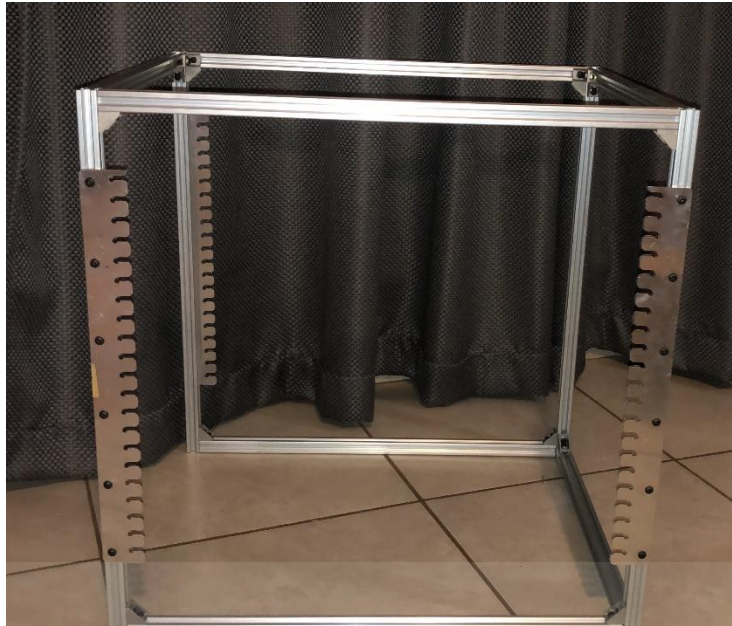
Figure 5.2: The frame of the EvoBot constructed using aluminium V-slot profiles. The height controls can also be seen in the figure.
