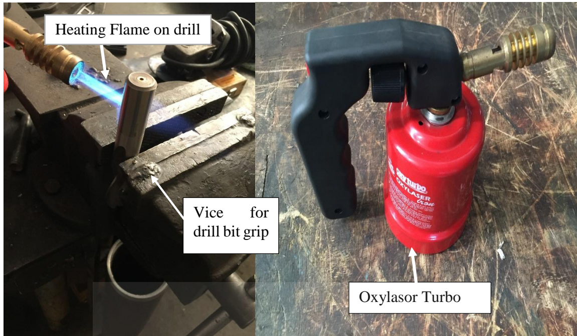
Figure 31: Drill preparation and heating
