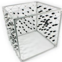
Figure 2: An acoustic camera capable of underwater operation [34]
