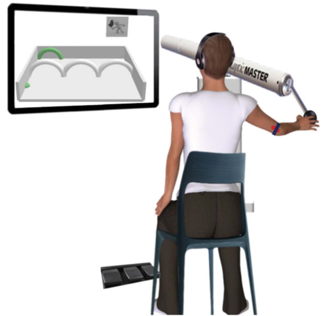
Figure 1. Experimental setup of the HapticMaster task with the participant seated in front of the LCD screen, the HapticMaster robot arm, and foot switch used to provide ratings of pain expectancy and fear of movement-related pain. Red dot and blue strap indicate electrode placement on the triceps tendon of the right arm for delivery of the e-stim (reprinted with permission from Meulders et al. 36 ).
