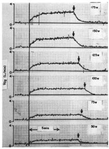
Figure 12 VO<sub>2</sub> of a subject during six constant-load exercises. Solid vertical line indicates the start of exercise. Arrows indicate the time exercise stopped. From Whipp and Wasserman 1972.
