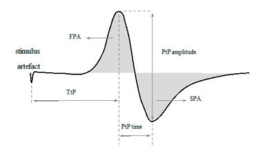
Figure 26. General representation of an M-wave and some of the commonly extracted parameters. Peak-to-peak amplitude (PtP), time between peaks (PtP time), time to peak (TtP), first peak area (FPA), second peak area (SPA). From Ibitoye, Estigoni et al.2014.
