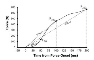
Figure 28 Common measurements of the rising force-time curve. Force at specific time points (F50, F100, etc.) and overlapping RFD measurement all starting from force onset the (RFD (0-50), RFD (0-100), etc.). Adapted from N.A. Maffiuletti et al. 2016
