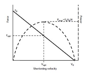
Figure 29 F-V relationship for a multijoint task. The linear solid line represents the linear F-V relationship; the dashed line represents the corresponding parabolic P-V. F0, force at null velocity; V0, velocity at null force; Pmax, peak power; Fopt and Vopt, optimal force and velocity for Pmax, respectively. From Jaric, S 2015.
