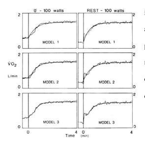
Figure 14 Best fits of single exponential models 1 (top), 2 (middle) and 3 (bottom) to averaged breath-by-breath responses of VO<sub>2</sub> to 100-W exercise from 0-W baseline (left) or from rest (right). From B.J. Whipp et al., 1982.
