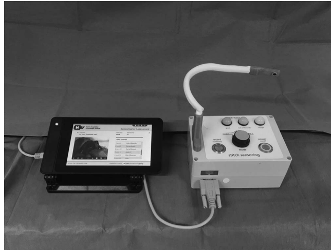
FIGURE 4. Overview of the supervision system, which comprises a user interface with a 12-in touch screen so as to review the procedure's recorded steps. This includes parameters that identify the trainee, date and time, and type or error (out of bounds, circumflex artery, coronary sinus, aortic valve, and conduction system). A control unit comprises an on-off button and a panel of lights to provide rapid feedback about the accuracy of the stitch when the trainee is passing it (a red light indicates danger, a blue light is used for out-of-bound stitches, and a green light reflects an appropriate stitch). A micro camera is mounted onto an articulated arm to film the surgical procedure.
