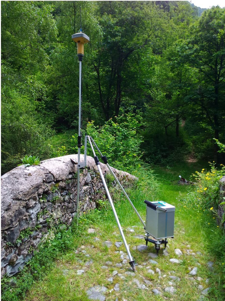
Figure 2.1 – A picture taken during a gravity field campaign. It shows the typical set up for a gravity measurement. On the left, the GNSS antenna recording satellite signals, for the a posteriori estimation of the point elevation. The antenna is usually placed as high as possible with respect to ground, to avoid the surrounding obstacles. On the right, the relative gravimeter on a tripod, used to level the instrument and usually sitting on stable ground, to avoid tilting and perturbations during the measurement.
