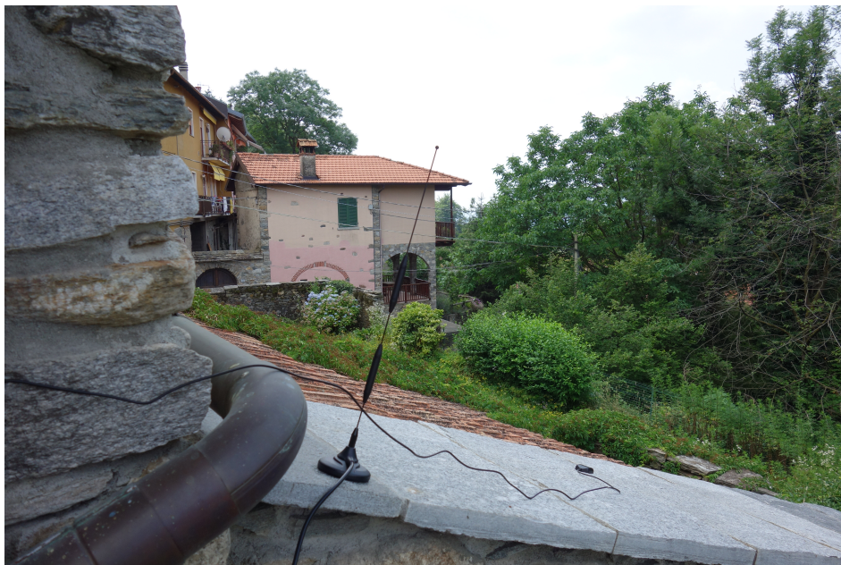
Figure 2.6 – Picture of the GNSS sensor (little black antenna on the right) which equipped every seismic station, to ensure a proper time synchronisation of the internal sensor clock. Next to it on the left, the mobile antenna for routine SMS notifications.
