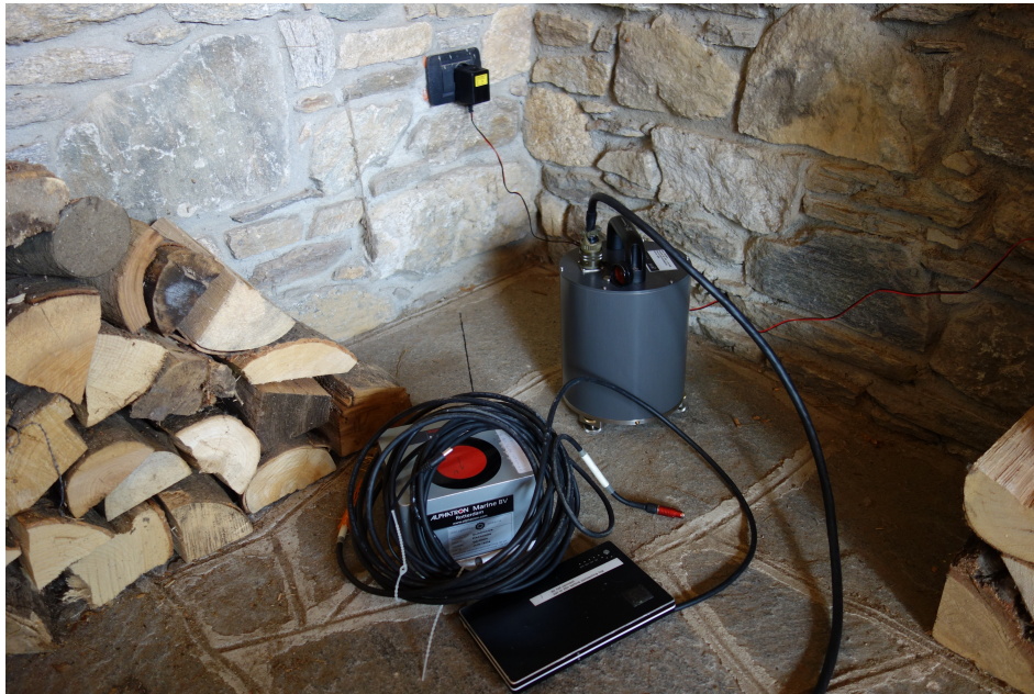
Figure 2.5 – Picture of the broadband seismic sensor IA06A installed in the framework of the IvreaArray seismic experiment, in the village of Cheggino.
