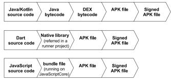
Fig. 2. APK build process.
