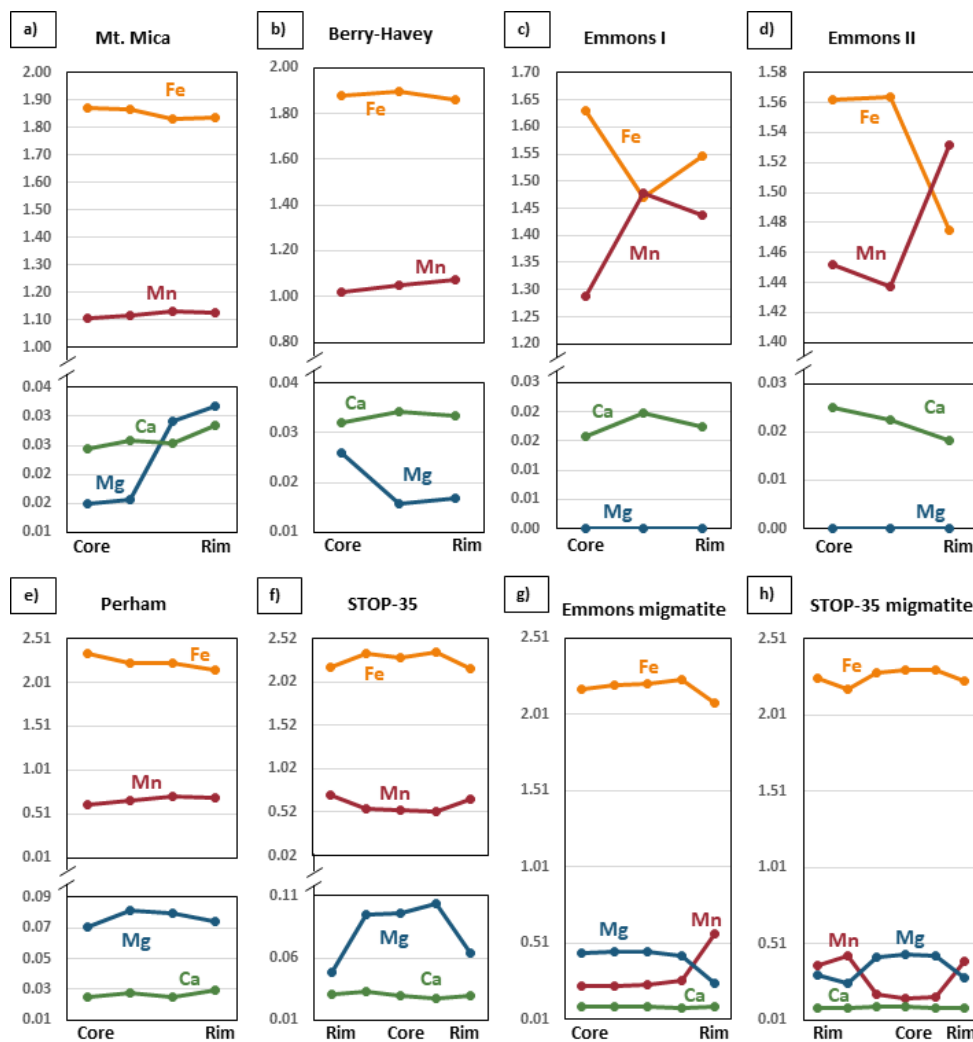
Figure 10. Major element variations across garnet crystals from the studied pegmatites (a–f) and migmatites (g,h). Values in cations (apfu).
