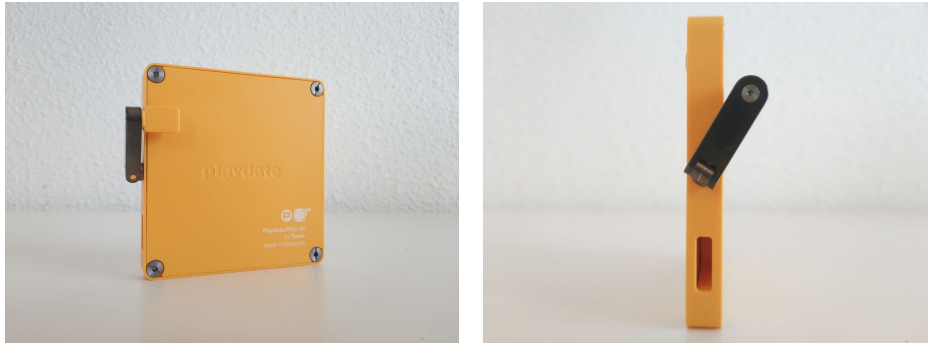
Figure 6.8: Collapsing the crank behind the device to create a switch interaction
