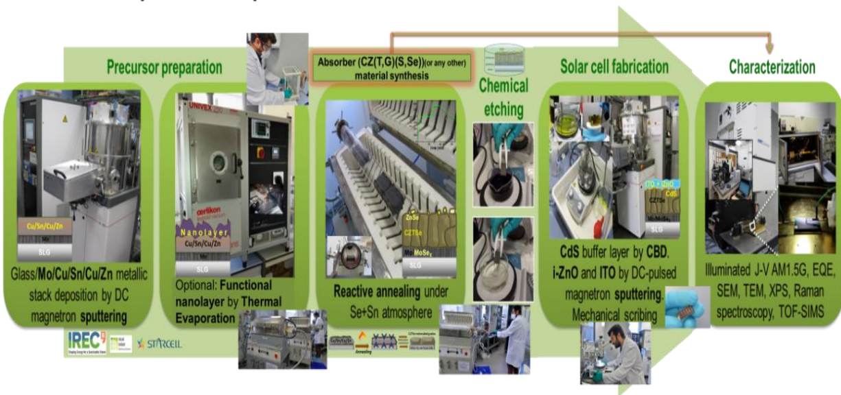
Figure 3.3.- Collage sketch for the general overview of the experimental solar cell device line processing steps followed during this Thesis.
