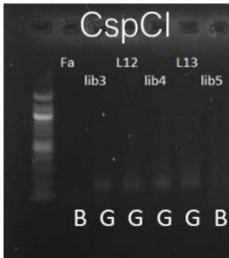
Figure S1. Example of library DNA quality identification. This agarose gel of C. caretta shows how library DNA was labelled as 'Good' (G) if the band was bright or 'Bad' (B) if the band was faint.
