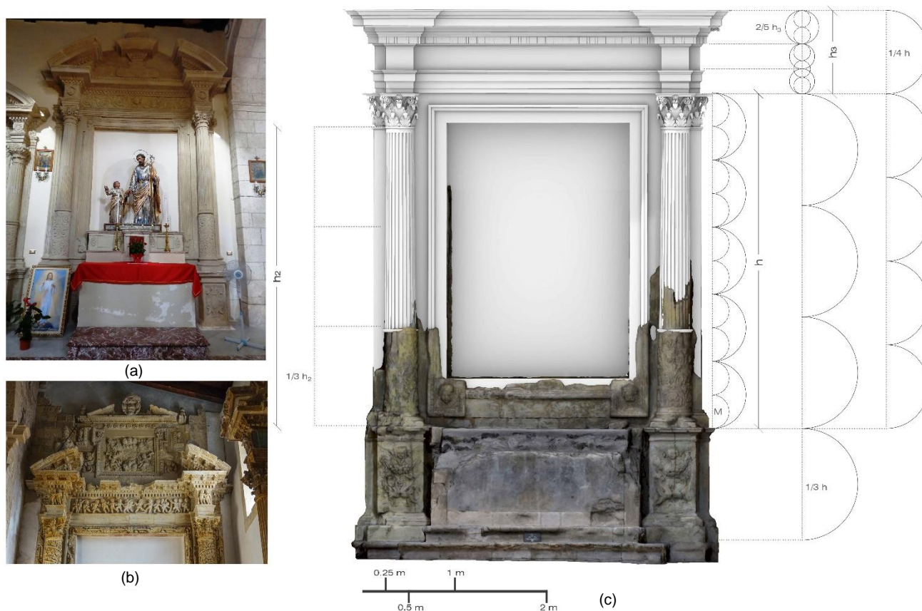
Figure 14: a) Altar of the Duomo of Condrò; b) Altar of Santa Maria la Vetere; c) 3D model of the altar of Crocifisso. In white, NURBS. In the original colours, photogrammetric mesh of the surviving parts.
