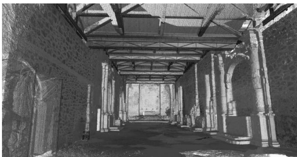
Figure 5: Laser scanner point cloud of the nave.
