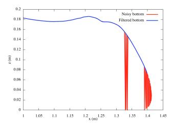
FIGURE 3. Illustration of the filtering process. Red line is the bottom after the extraction step. Blue line is the bottom after the filtering step.
