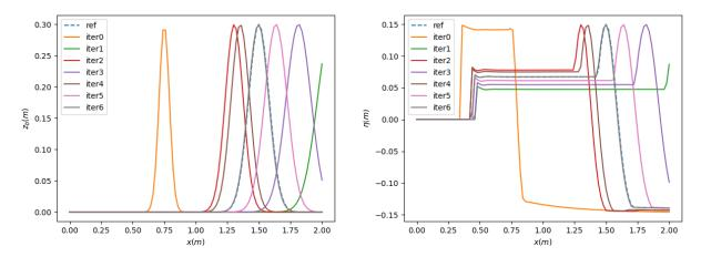
FIGURE 11. Evolution of the bathymetry (left graph) and the generated surface elevation (right graph) along time and iterations for the minimization problem of a Gaussian in translation.
