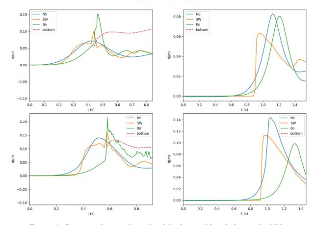
FIGURE 6. Comparison between the results of the three models with the same landslide size. The top line corresponds to the parameters (H,L) = (0.25 m, 0.45 m) while the bottom line corresponds to the parameters (H,L) = (0.45 m, 0.25 m). The left column corresponds to a probe at x = 0.75 m (wave generation zone) while the right column corresponds to a probe at x = 1.75 m (wave propagation zone).
