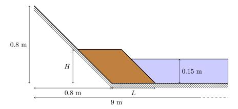
FIGURE 1. Initial state of the test case. The landslide is in brown and the water is in blue.
