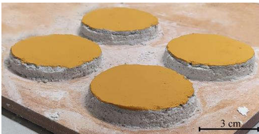
Figure 1. Laboratory developed wall painting specimens prior the consolidation.
