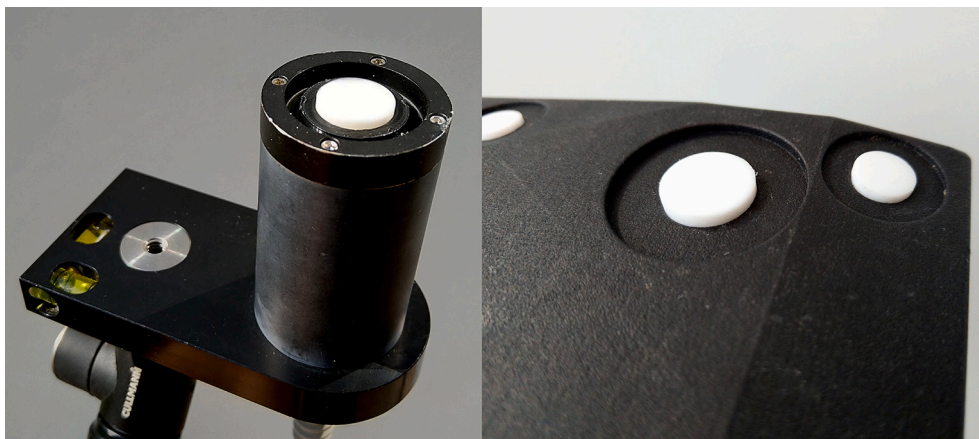
Fig. 7. (Left) The ASD FieldSpec RCR irradiance probe with the modification ring installed around the base of the diffuser. (Right) The improved FGI AIRS spectrometer and photodiode optics.
