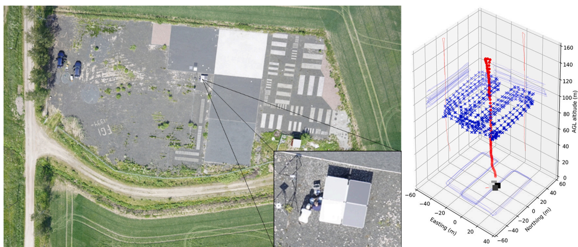
Fig. 5. (Left) An aerial image of the Sjäokulla test site with a zoomed in view of the reflectance reference panels. (Right) The GPS flight paths and image positions from the elevator flight (red circles) and a mapping flight (blue crosses) above the reference panels. (For interpretation of the references to colour in this figure legend, the reader is referred to the web version of this article.)
