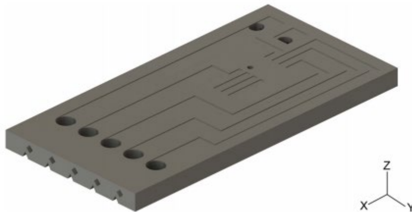
Figure 1. CAD model for the test articles. The outer dimensions of this part were 46 \times 23 \times 2.6 mm. The coordinate axes shown were used in the material extrusion machines.
