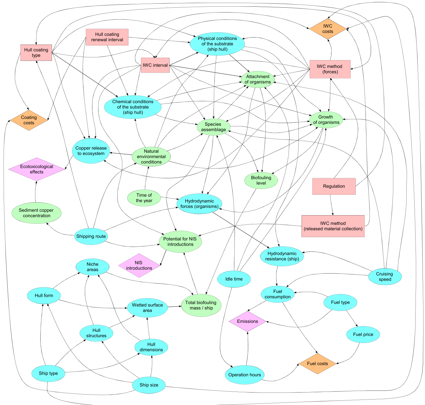
Fig. 4. The causal CID consisting of decision nodes (rectangles), chance nodes (blue ovals = technosphere factors; green ovals = ecosphere factors), utility nodes (orange diamonds = costs; purple diamonds = environmental impacts) and conditional dependencies (arrows) between them. When reading the CID, each arrow can be worded as “affect(s)”. A table explaining the meaning of each node is provided in Appendix IV. (For interpretation of the references to colour in this figure legend, the reader is referred to the web version of this article.)
