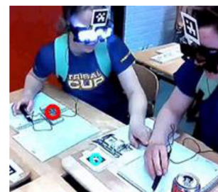
Fig. 4 Mobile gaze tracking gear and research setting. The light around the eyes in the picture is infrared light and invisible to the naked eye
