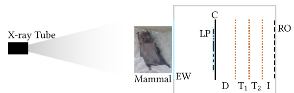
Fig. 1. Sketch of the experimental set-up, with a photograph of the mammal, the entrance windows (EW), the line phantom (LP), the cathode (C), the drift (D), transfer ( T i ) and induction gap (I), as well as the readout structure (RO).
