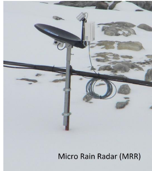
Figure 3. Micro rain radar (MRR) that will be deployed at Escudero station. Photo shows the same MRR model installed at Dumont d'Urville Antarctic station (France) during an APRES3 campaign in February 2017. ©Claudio Durán-Alarcón.
