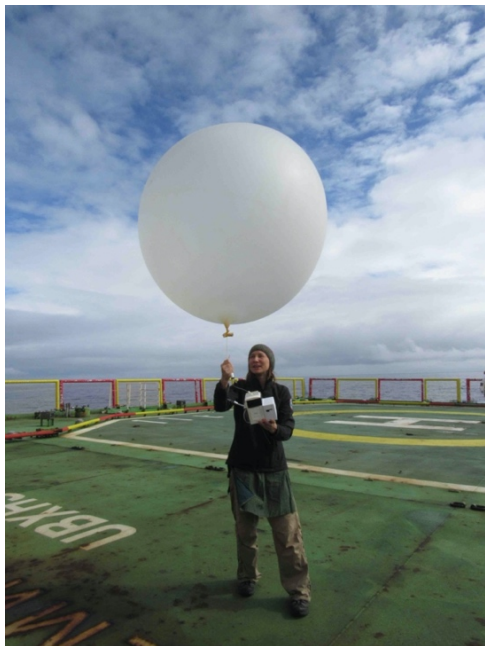
Figure 2: Launch of a radiosonde together with SLWC sensor during the Antarctic Circumnavigation Expedition. © Irina Gorodetskaya.
