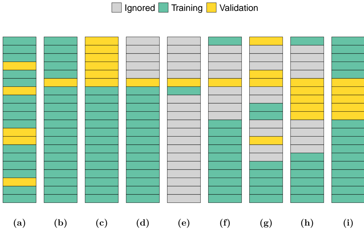
Figure 4.3: Various approaches to prediction error estimation. Columns represent one iteration of validation on temporally ordered data with first sample at the bottom and the last at the top. (a) k -fold CV, (b) Leave-one-out CV, (c) Fixed origin evaluation, (d) Rolling origin evaluation, (e) Rolling window evaluation, (f) h -block CV, (g) Modified CV, (h) hv -block CV, (i) Blocked CV
