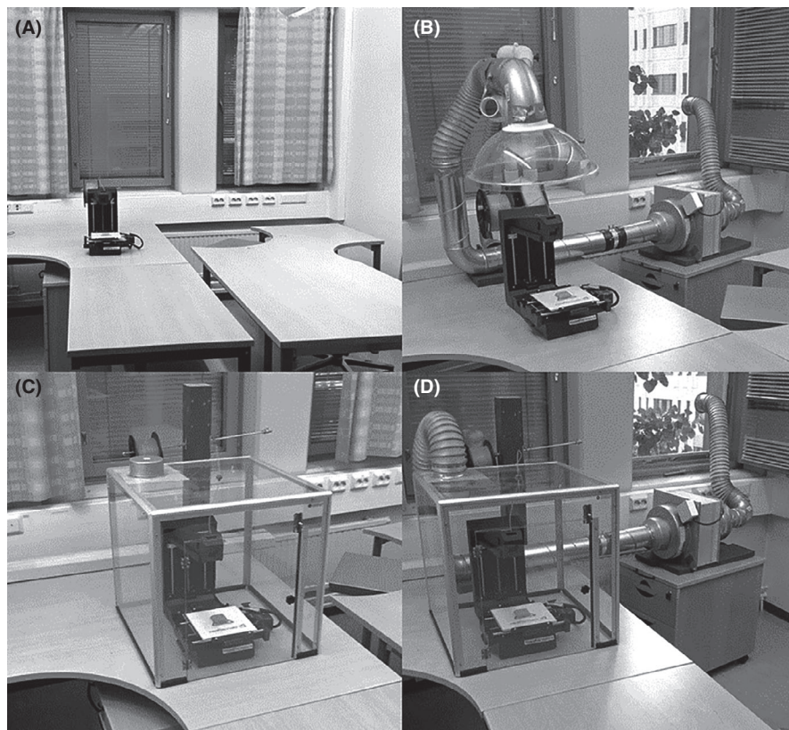
FIGURE 2 (A–D) The measurement setup with mechanical ventilation (A), local exhaust ventilation (B), enclosure (C), and enclosure with LEV (D)
